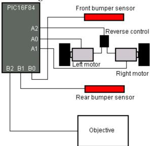
The diagram below gives details of the Input/Output connections for the buggy type envisioned in the component.
