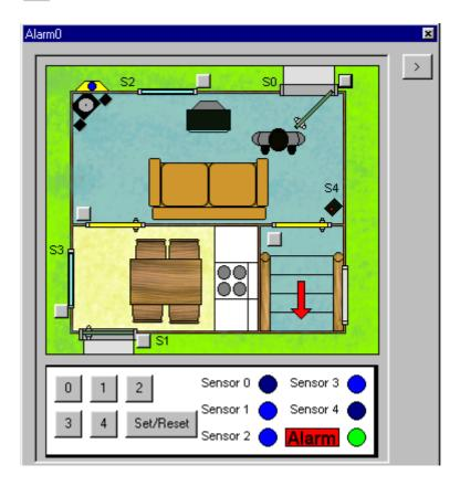
The component consists of a keypad and LED display to allow input and output, and a Virtual House in which you can open and close windows and doors to simulate the actions of an intruder.
