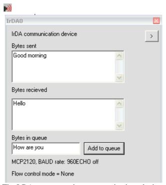
The IrDA component is a communications device used to communicate between the PICmicro and another IrDA equipped device.
