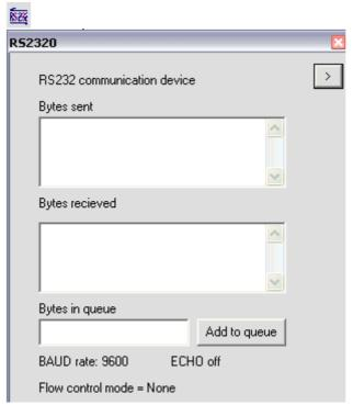
The RS232 component is a communications device used to communicate between the PICmicro and another RS232 equipped device.
