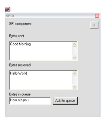
The SPI component allows the use of the SPI communications protocol in their programs.
