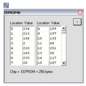
The EEPROM component allows users to write to and read from the EEPROM memory.
