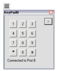
The Keypad is a 3 line 4 button matrix. To determine if a specific key has been pressed you can output a signal onto either the row that the key icon and check if there is a signal on the corresponding column. If there is then the button has been pressed making the connection.
