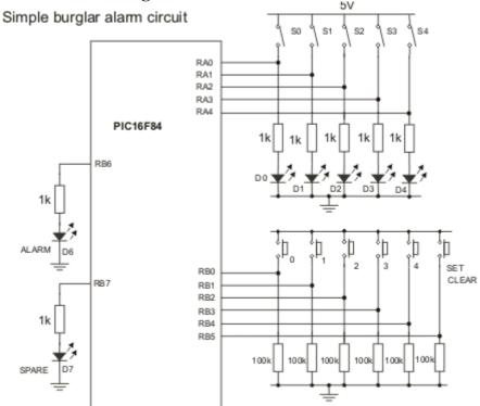
The circuit assumes a PIC16F84 chip is being used, adjust accordingly if another PICmicro microcontroller is being used.
